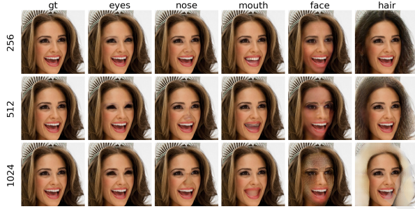
Figure 4: Restoring face key components at 256, 512, and 1024 resolutions using LaMa Model. The LaMa model faces challenges in restoring effectively at resolutions higher than 256. View better when zoomed in.
